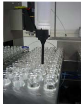
Overhead gravimetric addition of solid while mixing, heating and cooling
